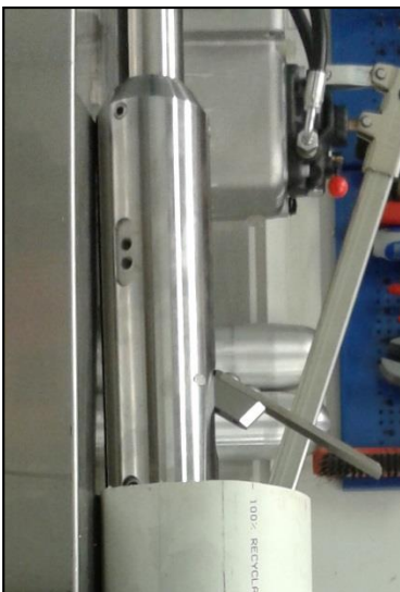
Holelock arm for steel casing with pump in background
