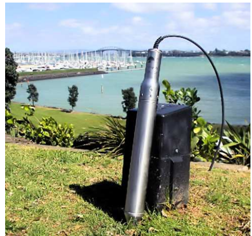
An example of a borehole seismometer manufactured by IESE Ltd
